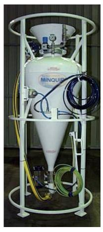
We have produced a range of "Anfo Pressure Loaders" from 25kg to 500kg capacities.
